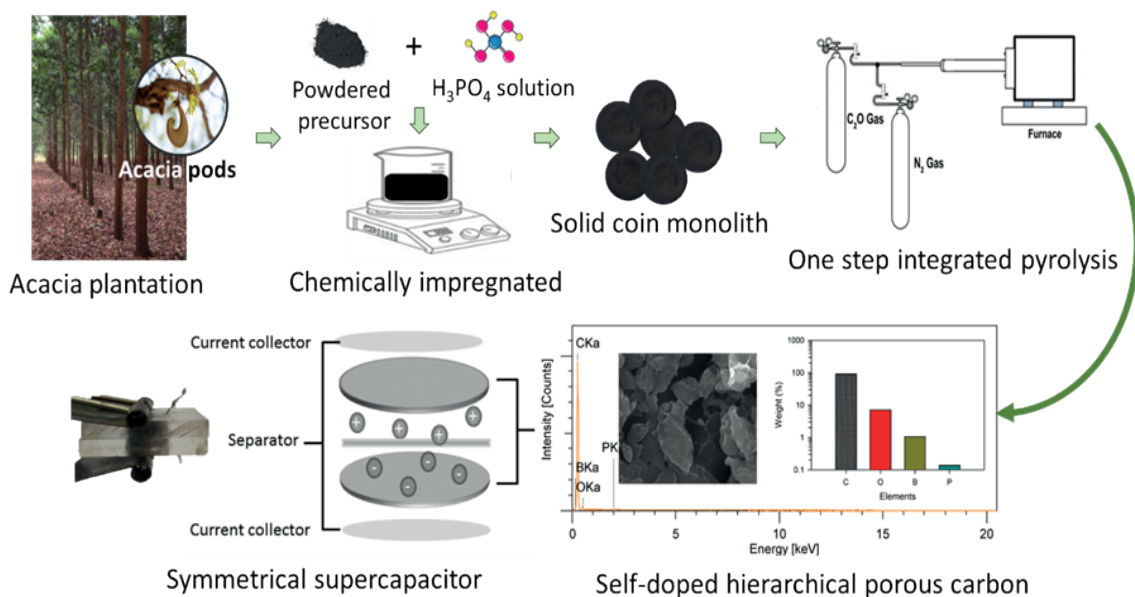
Figure 1. Schematic representation of doped porous carbon produced from acacia plantation residues (acacia pods).
