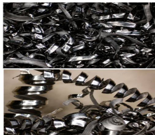
Figure 16. Segmented chip formation during the machining of a titanium alloy [176].
