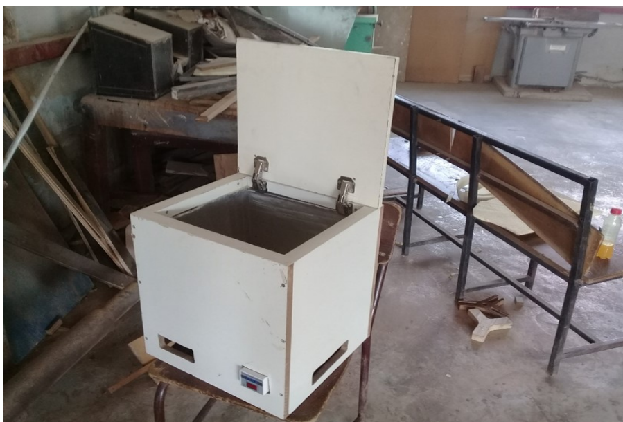
Fig. 4. Image (Isometric view) of Fabricated Deep Freezer
